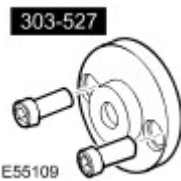
Crankshaft rear oil seal installer 303-527
